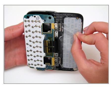
Gently peel the clear plastic keyboard backing off of the keyboard. It is attached to the keyboard by a weak adhesive.
