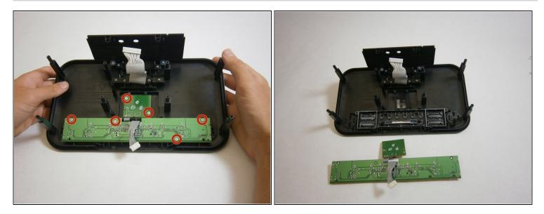
Use a Phillips #000 screwdriver to unscrew six, 5 mm-length 5 mm-head, screws attaching the buttons to the case.
