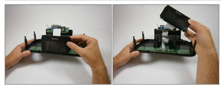
• Gently push the screen away from you to dislodge it from the plastic clip holding it in place and then pull up to remove.
