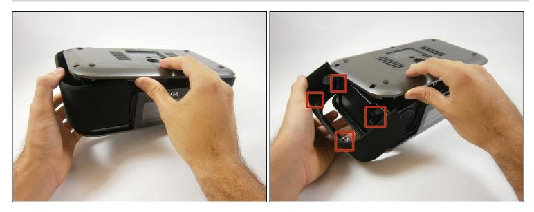
A Potential for device damage: Be careful not to use too much force or you might break the plastic rings holding the side panels in place.
