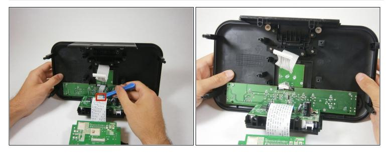
Use a plastic opening tool to pry and lift up the white zip connector attaching the LCD screen to the buttons.
