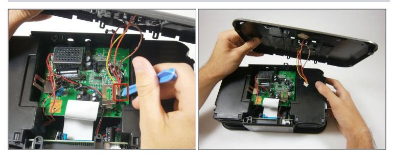
• Use a plastic opening tool to pry off the white ZIF connector joining the wires to the motherboard.
