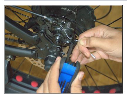
Tighten up the bolt while you keep pulling the cable.
