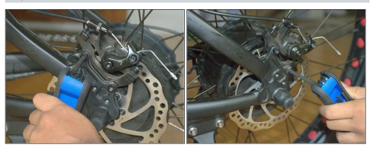
To center the caliper for a smooth breaking experience, loosen up the two bolts of the brake situated at top and at bottom.
