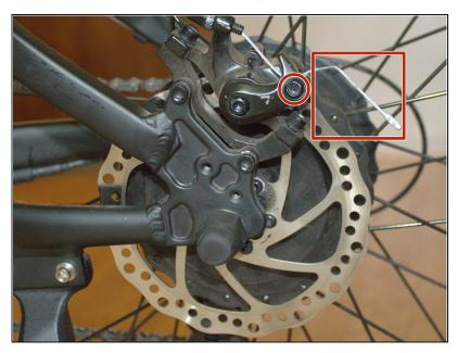
i You will see a cable attached to an Allen bolt.
