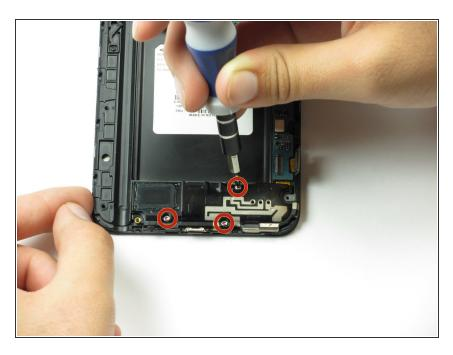
Remove the three 3mm screws on the bottom of the device with a Phillips #00 screwdriver.
