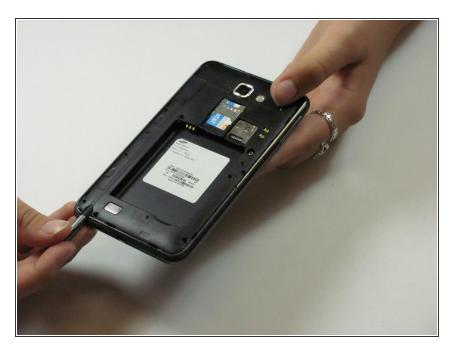
Remove the stylus from the bottom of the phone.
