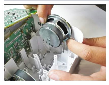
Pull up on the metal brackets, found on either side, until the speaker is completely removed. Removing the speaker is rather challenging. Don't get discouraged if it takes multiple attempts!
