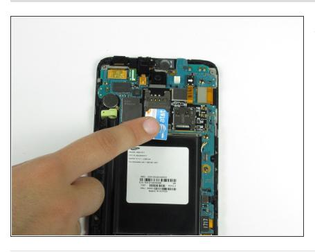
Pull out the (white and blue) SIM card directly above the empty battery slot.
