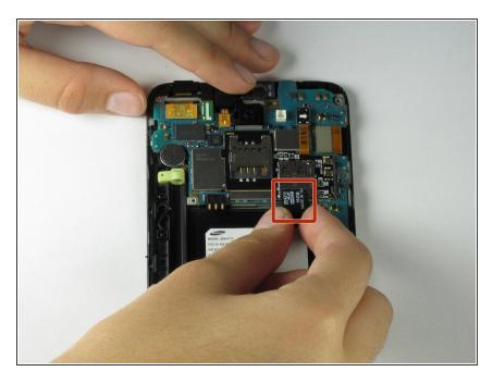
Pull out the micro SD card located in the upper right slot (above the battery).
