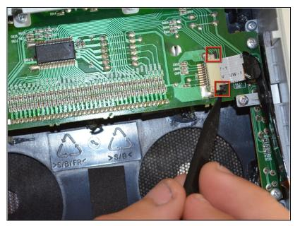
Remove the ribbon cable from the ZIF connector by pulling out the two black tabs with the pointed end of the spudger then pulling the cable straight out of the connector.
