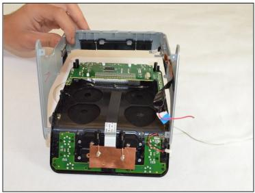
Remove the grey side piece from the black front panel by pulling it straight up. It should easily slide off.
