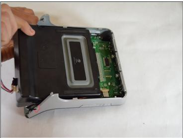
Slide the speaker towards the bottom of the device to remove.
