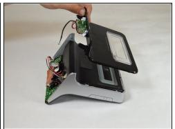
• Slide the back panel towards top of the device and lift away from the device to detach back panel.
