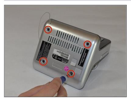
Gently unscrew the four 15.5 mm Phillips #2 screws that hold the bottom panel to the dock.
