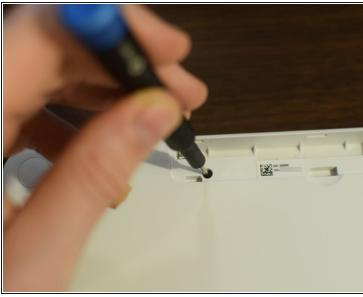
Use a Phillips #0 driver to remove the two black screws that were covered by the battery compartment
