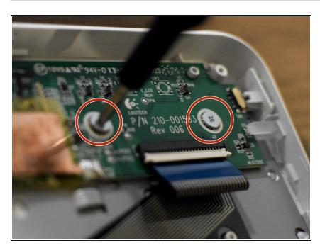
Use a Phillips #0 driver to remove the two screws holding down the logic board, on either side of the cable connector.
