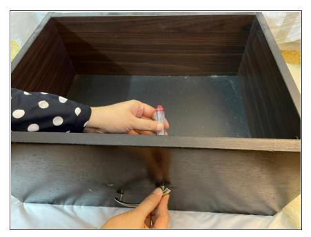
• Tighten the good side of the handle by rotating the screwdriver in a clockwise direction.
