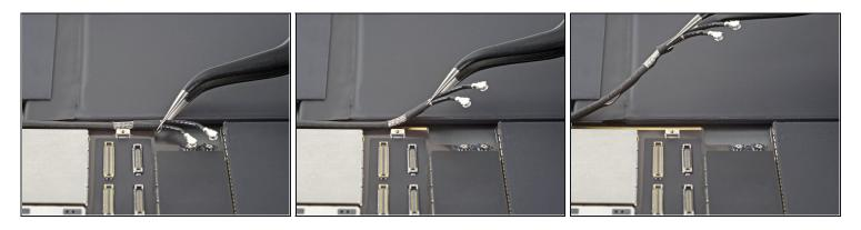
• Use a pair of tweezers to lift the antenna cables away from the logic board.
