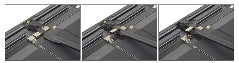
• Insert an opening pick or a halberd spudger underneath the front camera to cut the adhesive securing it to the rear case.
