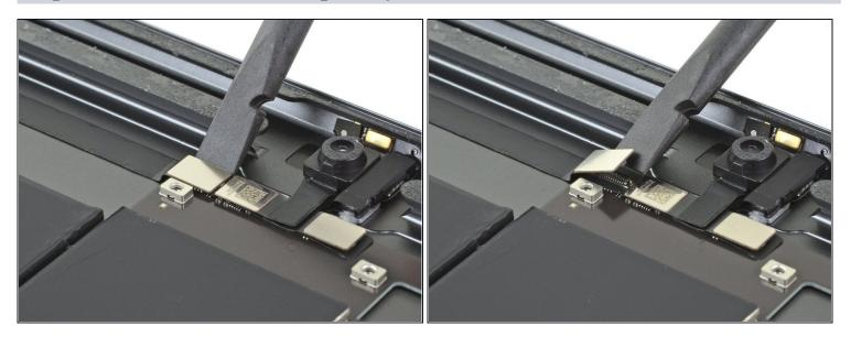
• Use the flat end of a spudger to disconnect the headphone jack cable by lifting straight up on the press connector.
