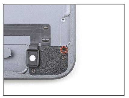
• Use a Phillips screwdriver to remove the 2.8 mm-long screw securing the headphone jack to the rear case.
