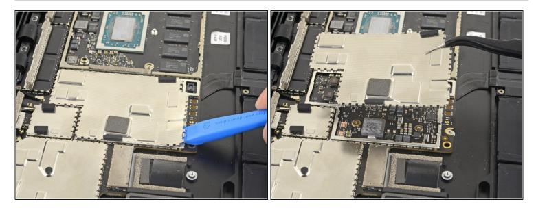
Repeat the previous step to remove the second shield from the left side of the motherboard, closest to the CPU.
