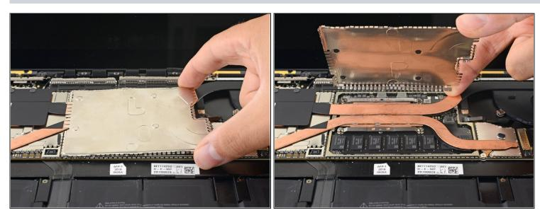
• Remove the heatsink shield.
