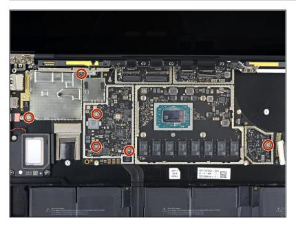
Use a T3 Torx driver to remove the six 2 mm screws securing the motherboard.
