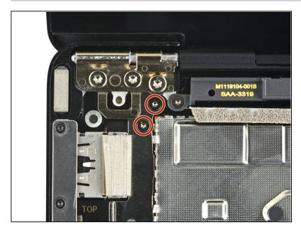
Use a T3 Torx driver to remove the two 3 mm screws securing the motherboard bracket.
