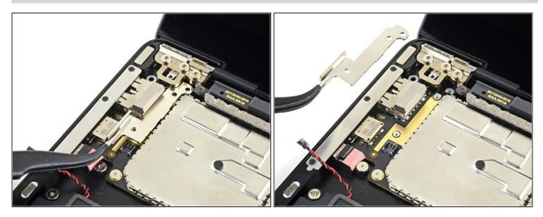
Use a pair of tweezers to remove the motherboard bracket.
