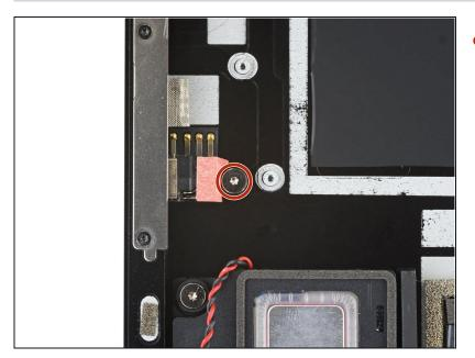
Use a T3 Torx driver to remove the 2.6 mm screw securing the headphone jack.
