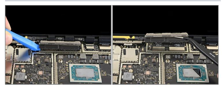
Repeat the previous step to remove the remaining shield from the left bank of display connectors.
