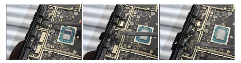
Disconnect the three remaining display connectors.
