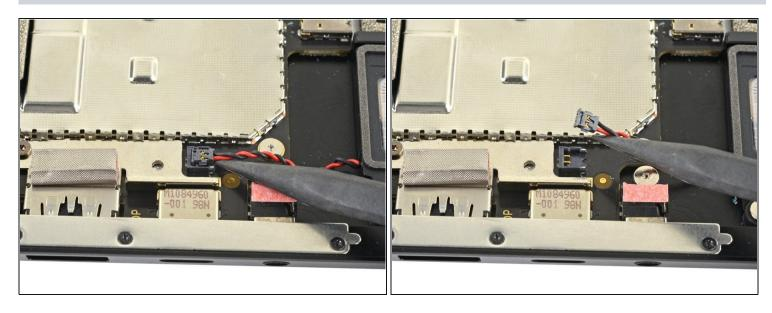
Use the pointed end of a spudger to lift and disconnect the left speaker wire from its connector on the motherboard.
