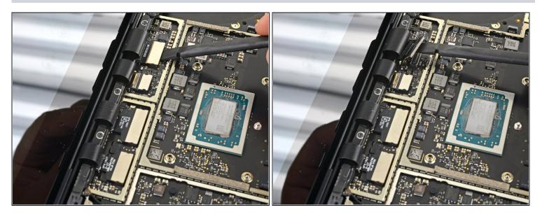
Use the flat end of a spudger to pry the first display cable up and out of its socket on the motherboard to disconnect it.
