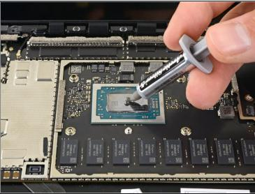
Before reinstalling the heatsink, follow this guide to clean the heatsink and CPU and reapply thermal paste.
