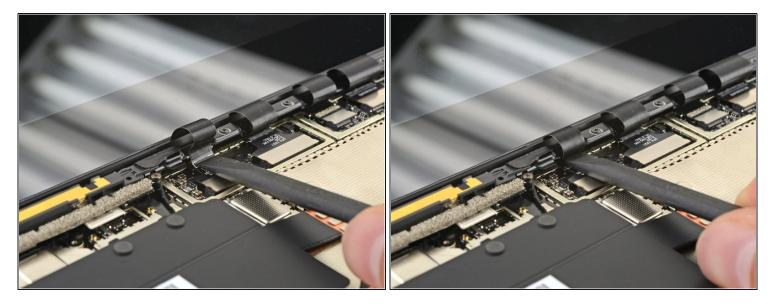
During reassembly, use the flat end of a spudger to gently push the display cables back into their cavity in the lower case.
