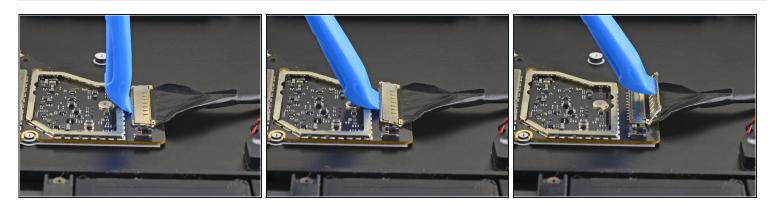
Use an opening tool to flip open the gold locking arm on the Surface Connect port's motherboard connector.
