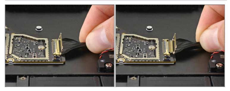
• Grip the Surface Connect port cable and pull it away from its connector to remove it.
