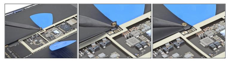
Use a spudger to move the Smart Connector cable behind the opening pick.
