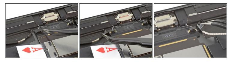
Use a pair of tweezers to remove the tape from the back of both speaker connectors.
