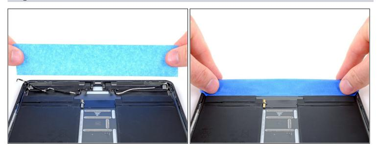
Cover the lower components with a strip of tape.
