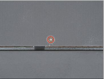
• Use a Phillips screwdriver to remove the 1.3 mm-long screw securing the logic board shield.
