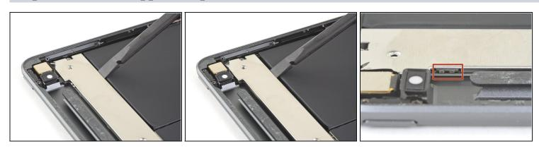
• Use a spudger to push the upper component bracket towards the upper edge and off of the clips located near the rear camera.
