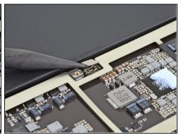
Use the pointed end of a spudger to disconnect the Smart Connector cable by lifting straight up on the press connector.
