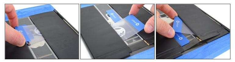
Use the adhesive remover and the opening cards to loosen the remaining battery adhesive strips.
