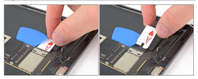
• Remove the battery blocker.
