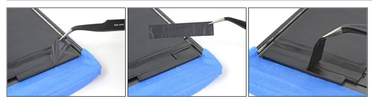
• Use a pair of tweezers to remove the two pieces of tape securing the battery to the lower buffer blocks.
