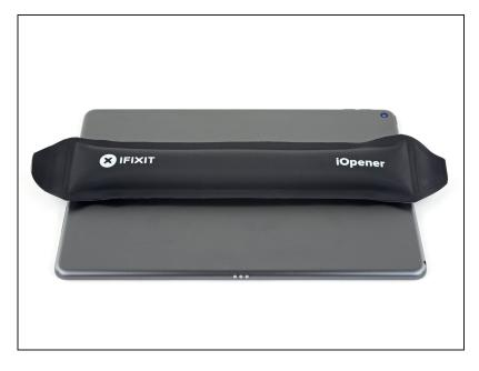
Apply a heated iOpener lengthwise down the center of the rear case to soften the logic board adhesive.
