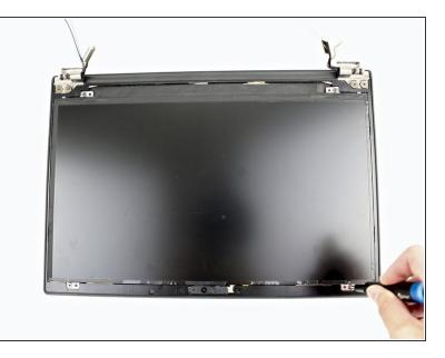
Remove four 2.9 mm screws from the LCD panel using the Phillips #1 screwdriver.
