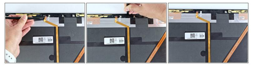
Use a spudger to pry the camera up from the LCD Unit.
