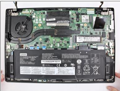
Remove all antenna cables from their routing.
