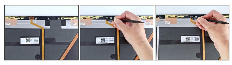
Using a spudger, disconnect the cable from the camera.
