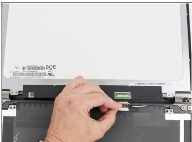
Remove the LCD cable from the socket.
