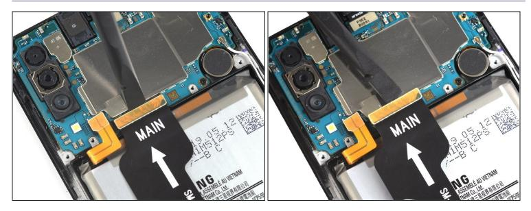
• Use a spudger to disconnect the interconnect cable from the motherboard by prying the connector straight up from its socket.
