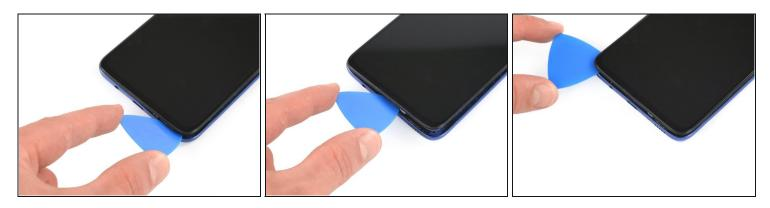
• Continue sliding the opening around the bottom right corner to the bottom left corner to detach the plastic clips.
