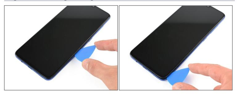
• Slide the opening pick to the bottom right corner to detach the plastic clips.
