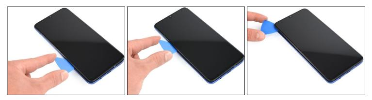
Slide the opening pick along the left edge to detach the plastic clips.
