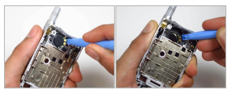
• Use the opening tool to lift the speaker out from the right side.
