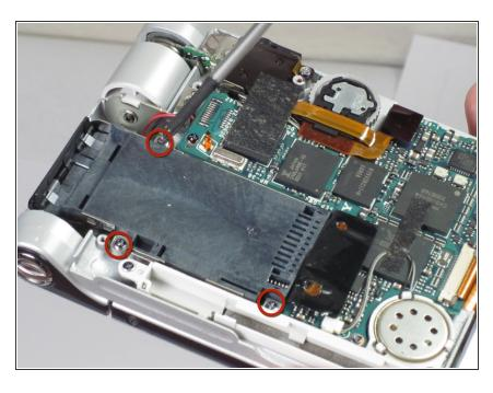
Holding the memory module in place, unscrew the three 0.9mm screws with a Phillips #00 screwdriver.
