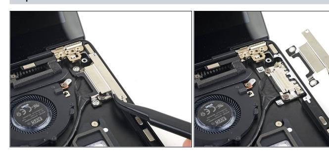
Remove the Surface Connect port cover.
