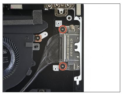
Use a T3 Torx driver to remove the two 3 mm screws securing the Surface Connect port.
