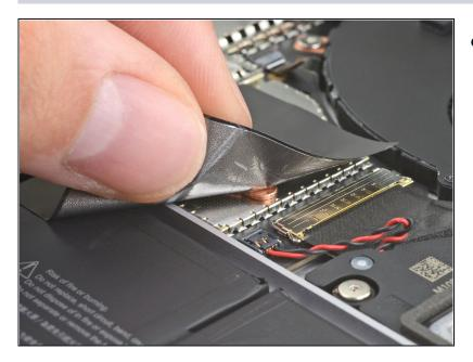
Use your fingers to peel back the black tape covering the right speaker and Surface Connect port connectors.
