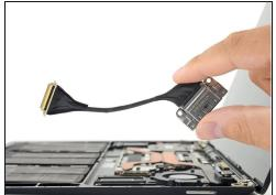
Pull the Surface Connect port away from the edge of the chassis to remove it.
