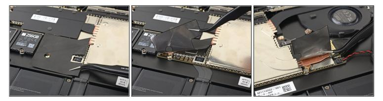
• Use a pair of tweezers to remove the two pieces of black tape covering the bottom left and bottom right corners of the motherboard.
