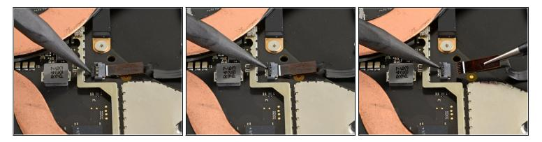
• Use the pointed end of a spudger to flip up the locking flap on the fan cable's <u>ZIF connector</u>.
