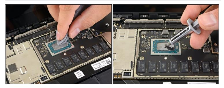
Before reinstalling the heatsink, follow this guide to clean the heatsink and CPU and reapply thermal paste.
