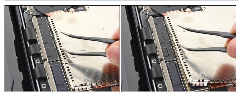
• Continue along the heatsink's top edge, inserting a tweezer arm into the shield holes and prying upwards on each one as you go.
