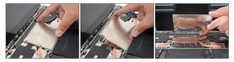
• Once the top edge is loose, use your fingers to grip the top of the shield and pull it up and away from the heatsink to release the remainder of the shield.
