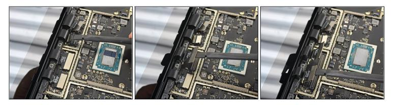
Disconnect the three remaining display connectors.
