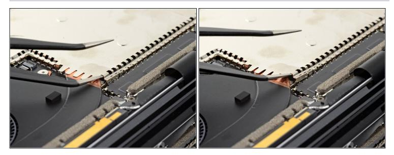
Repeat the previous step's procedure to release the top right corner of the heatsink shield.
