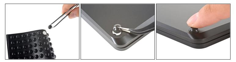
In place of reusing old, worn out feet on your device, 8 mm rubber furniture pads can be a good substitute.
