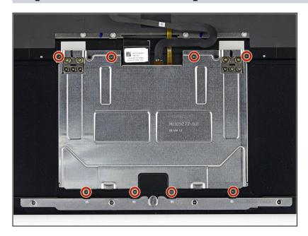
• Use a T3 Torx driver to remove the eight 2 mm screws securing the touchpad cover.
