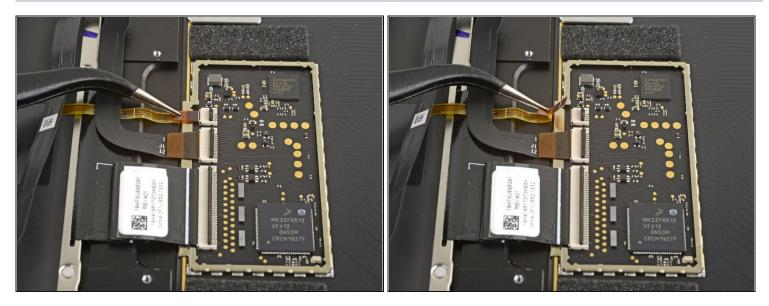
Use a pair of tweezers to slide the first ribbon cable out of its connector.
