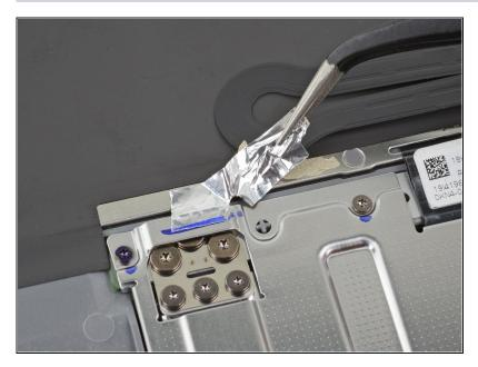
• Use a pair of tweezers to remove the two pieces of metallic tape covering the top edge of the touchpad cover.
