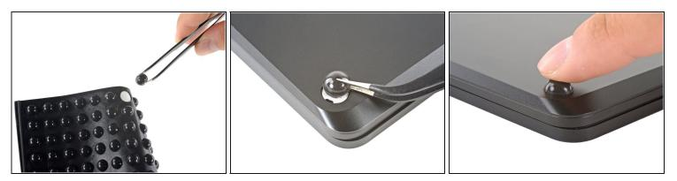
In place of reusing old, worn out feet on your device, 8 mm rubber furniture pads can be a good substitute.
