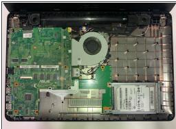
Carefully remove the battery using a plastic opening tool.
