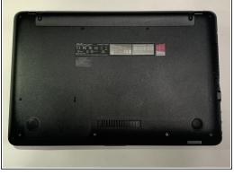
Use a Phillips #00 screwdriver to remove the ten 1.2 mm screws attached to the back cover of the laptop.
