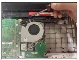
Remove the two 1.2 mm screws holding the battery in place using the Phillips #00 screwdriver.
