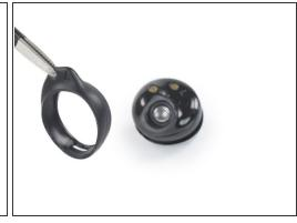
Use your fingers or a pair blunt nose tweezers to remove the earbud's rubber wingtip by pulling it upwards while slipping it off the earbud.
