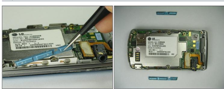
• Use tweezers to remove the volume control buttons on the opposite side of the phone.
