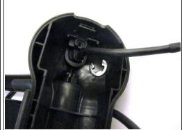
Wedge the pointy end of the spudger between the sliver E-ring and USB attachment base to extract the E-ring and release the USB cable.
