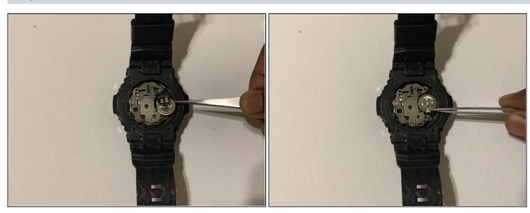
• Slide the new battery into the frame and bend the metal guide onto the battery.
