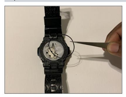
Use the tweezers to remove the rubber gasket by lifting it.
