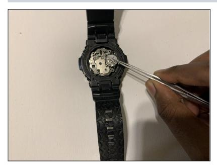
Peel off the protective sticker from the surface of the old battery.
