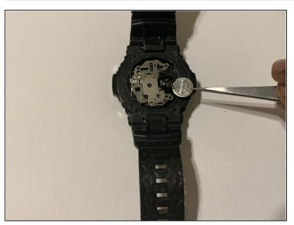
Remove the old battery from the guide with tweezers.
