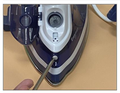
• Push the spray nozzle using the pointed end of a spudger.
