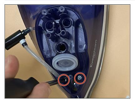
Remove the two screws using a Phillips #0 screwdriver.
