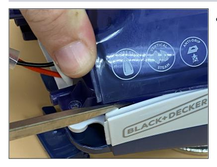
• Rotate the spudger so that it separates the top of the white plastic from the bottom of the purple plastic.
