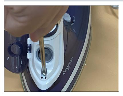
Remove the single screw located under the rubber cover using a Phillips #0 screwdriver.
