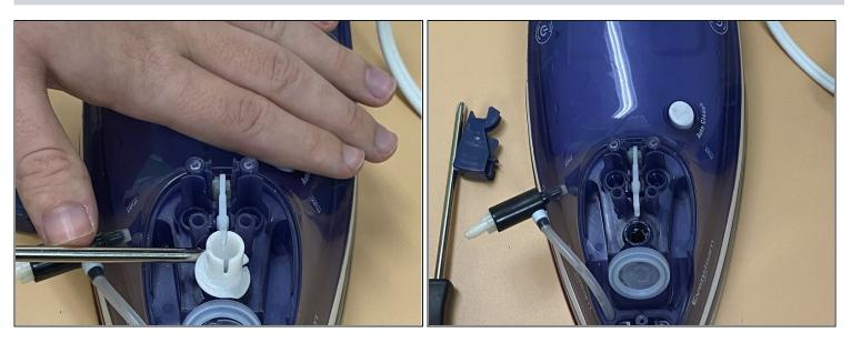
• Pry the white plastic cylinder out from its hole using a spudger.
