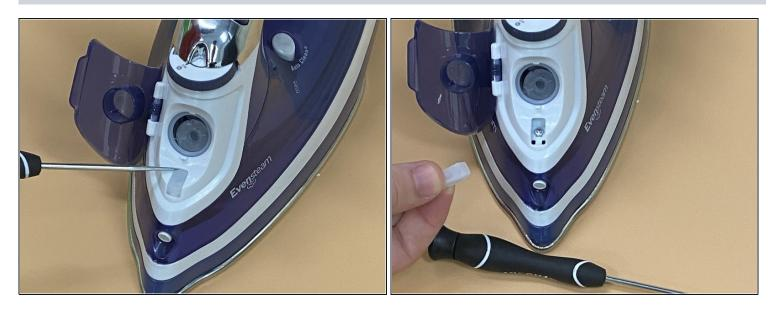
• Use a spudger to remove the clear rubber cover from the front of the iron.
