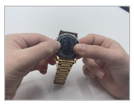
Press firmly on the battery cover, using both of your thumbs to snap it back in place.
