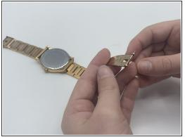
• Re-insert the pin you removed into the hole of the smaller (lengthwise) folding segment.
