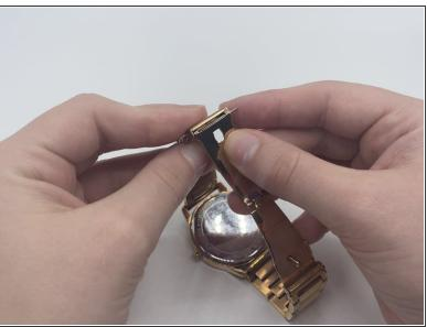
Align both ends of the watch, holding the segment with the spring pin adjacent to the hole.
