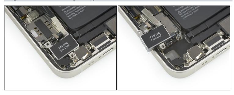
• Use a pair of tweezers to remove the Taptic Engine.
