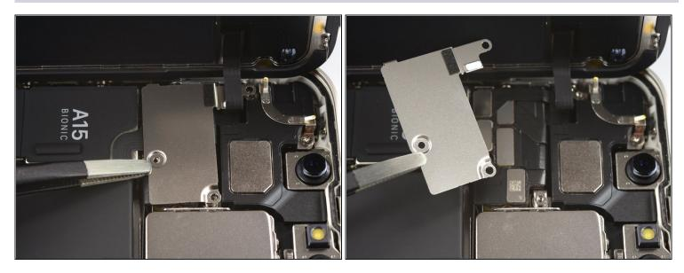
• Use a pair of tweezers to remove the front sensor assembly connector cover.
