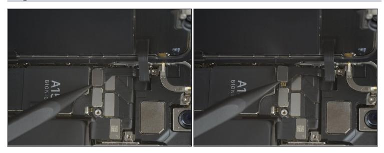
• Use a spudger to disconnect the front sensor assembly cable connector.
