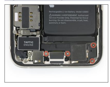
• Remove the four 1.5 mm-long Phillips screws securing the speaker.
