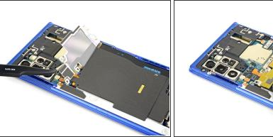
Use a pair of tweezers to lift up and flip back the metal shield covering the battery connector.
