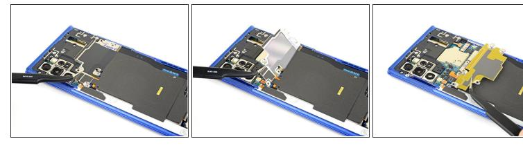
Use a pair of tweezers to lift up and flip back the metal shield covering the battery connector.
