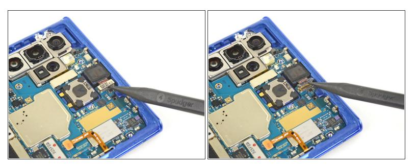
• Use the pointed end of a spudger to pry the front-facing camera connector straight up from the motherboard.
