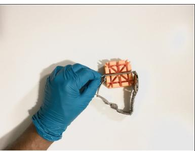
Align the link pins to be added on the holes that connect the desired link to the wristband.
