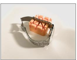
Lay and secure the wristband on the watchband holder.
