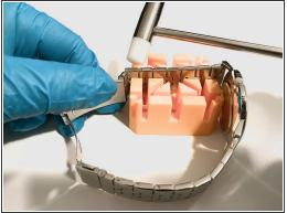
• Use the hammer to gently tap the link pins into the holes until the pin is completely resting in position.
