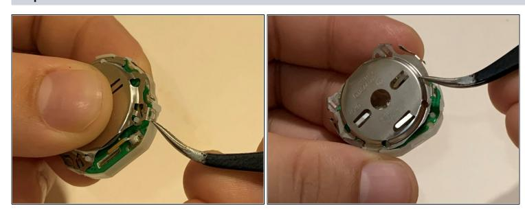
• Use a pair of tweezers to lift the metal clasps at each corner and remove the battery holder.
