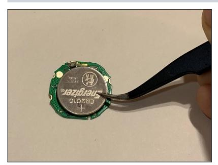
Attach the battery to the new circuit board.
