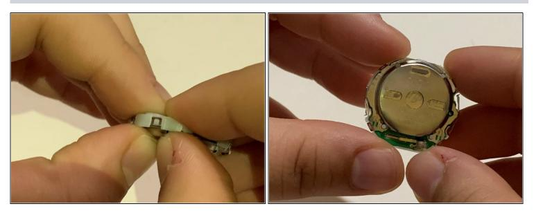
Reattach the battery holder and push down on the clasps at each corner.
