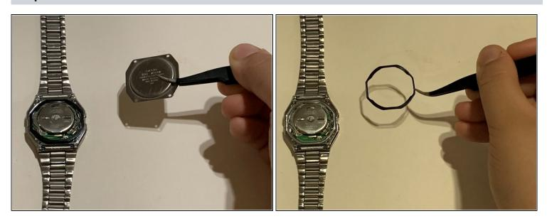
Remove the back cover and the black rubber band with tweezers.
