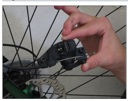
After removing the bolts pull of the brake caliper from the brake disc.
