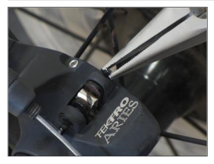
Bend the retention pins straight using a pair of needle nose pliers.
