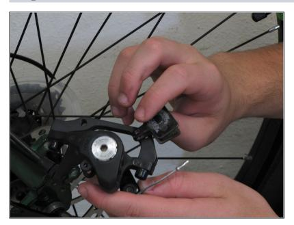
Remove the brake pads by pulling on them and realesing them from the caliper.
