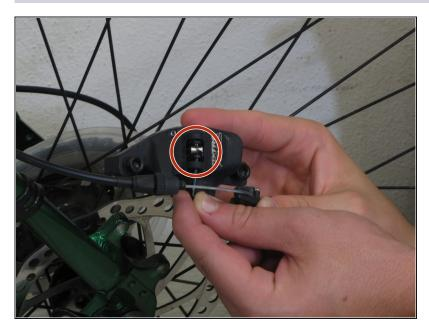
Using the needle nose pliers remove the retention pin by pulling on it.
