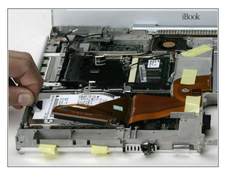
• Peel back the black tape to free the microphone cable from the hard drive.
