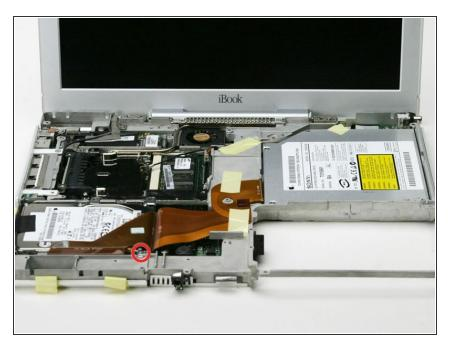
• Remove the single Phillips screw to the right of the hard drive connector.
