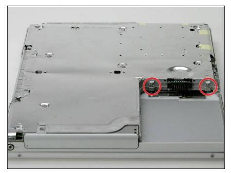
• Remove the small greasy springs with white plastic caps from either side of the battery contacts.
