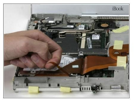
At the front edge of the hard drive, lift up on the transparent orange tape to disconnect the ribbon cable from the main board.
