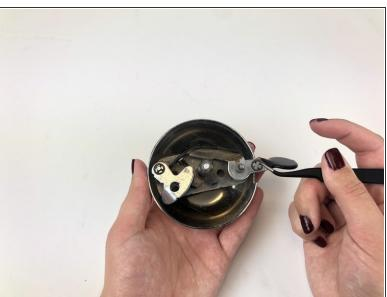
Use the tweezers to gently bend up the prongs on the metal four-pronged rings.
