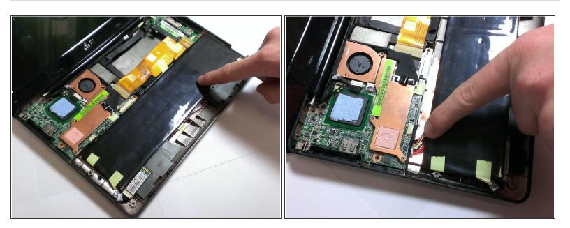
Use your fingers to lift the battery and gently disconnect the wires from the base.
