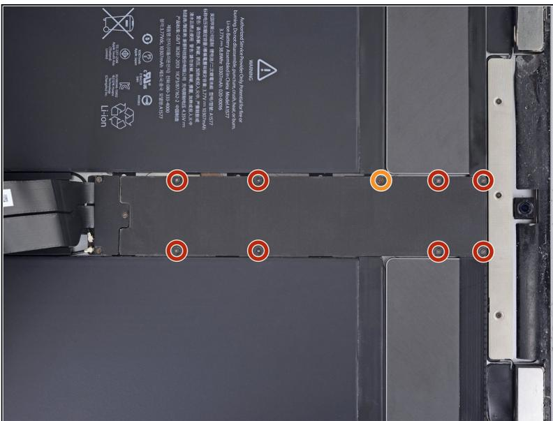
⚠ It's important to disconnect the battery before you proceed further. Detaching or connecting the display cables with the battery plugged in can cause a short that will destroy touchscreen functionality.
