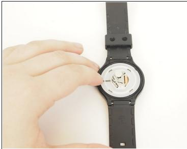
• If the rubber seal pops out, realign the rubber seal with the groove along the back face.
