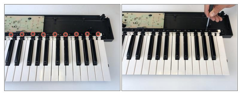
• Remove all the 10 mm screws on the top of the keys using a Phillips #1 screwdriver.
