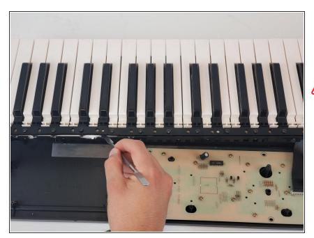
Use a spudger to separate the teeth to the plates that hold the keys together.
