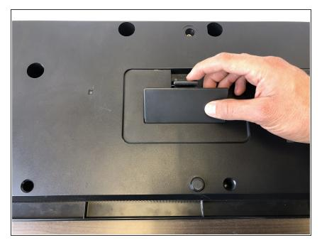
• Pull the tab and remove the battery cover.
