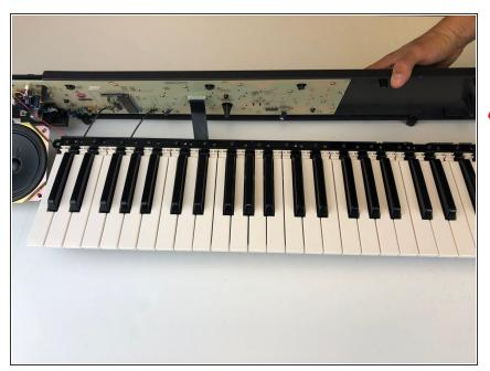
• Lift the front plate of the keyboard and rotate it 180°.
