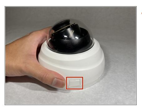
Press down on the side button, and lift up the top dome.
