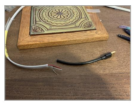
Figure out what length of new USB cable you want and cut it to that length. Leave a few extra inches in case you cut the wires while striping
