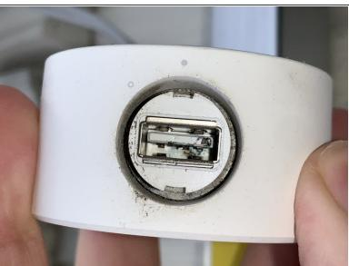
• The Nest Outdoor Camera (not to be confused with the Nest IQ Outdoor Camera) gets power through a long USB cable that connects to a power adapter, which connects to an outlet. The USB connector is not as waterproof as advertised, and this one got wet, became corroded, and the camera stopped working.
