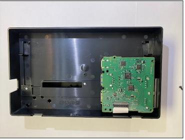
• Carefully pull to remove the backing from the switch dock, exposing the circuit board.
