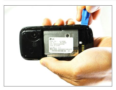
• Use a plastic opening tool to pry the rear case loose.
