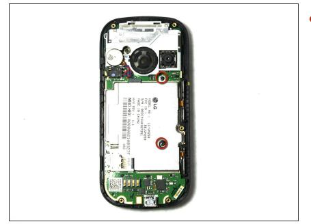
Remove the two 2.9 mm Phillips #000 screws that are slightly offcentered to the right.
