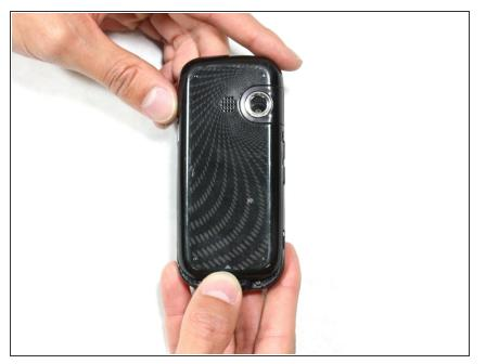
• Apply an upward force to slide the back cover off.
