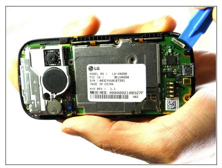
• Use the plastic opening tool to pry the motherboard loose.
