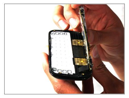
Once the motherboard is lifted, rotate the motherboard up 90 degrees to the right.
