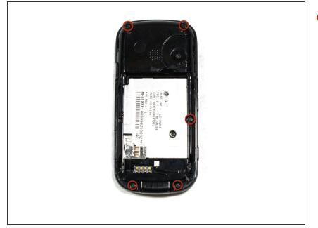
Remove the five 3.0mm Phillips #000 screws along the edge of the rear case.
