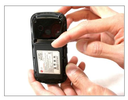
• Use your finger to push down on the top of the battery and pull it out.
