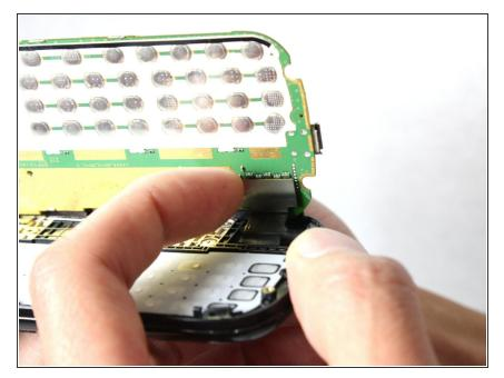
• Use your finger to pull the flex cable out from its connector.
