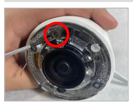
Remove the four small screws from the plastic camera cover.
