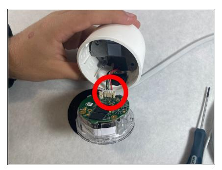
Disconnect the microphone cable to separate the motherboard from the main camera unit.
