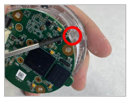
Pry the plastic cover away from the motherboard at the plastic clips using a spudger.
